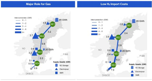
Figure 35 – Hydrogen infrastructure in 2045, Sensitivity 1, Low H<sub>2</sub> import costs
