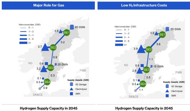
Figure 37 – Hydrogen infrastructure in 2045, Sensitivity 2, Low  $H_2$  infrastructure costs
